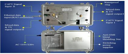
The output of the Master is the coaxial output with mixed Video and data services. The following figure shows the ports configuration of EoC master.
