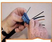
Cutting loose tube with tube cutter
